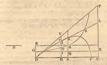
let DA: AC:: resistance: gravity. Also DP: CP:: resistance: gravity,  $\therefore$  DA×DP: CP×CA:: R: G. Between DC, CP describe a hyperbola sutting DG and AB perpendicular to DC in G and B, from R draw RV perpendicular cutting DP in V and the hyperbola in T, complete the parallelogram G K CD and make N: QB:: CD: CP.
